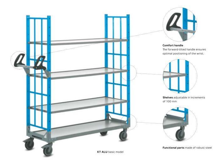
**Standard equipment:** side panels, shelf frames and chassis frame made of aluminium. 3 shelves with platform made from aluminium-plastic composite material, can be bolted on at 100 mm intervals. Ergonomic comfort handle. Functional parts made of steel for optimum stability.
